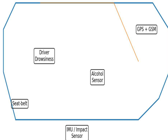
Fig. 2. Representative sensor placement in a passenger vehicle.
